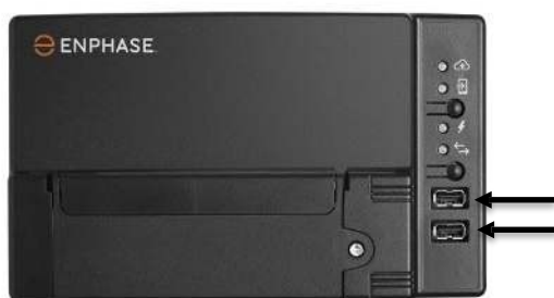
Microinverter Communications LED Device Scan button
